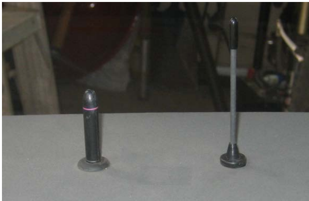
Figure 1 Example of factory installed glare shield antennas; required ground plane is hidden under the cover. ADS-B/SSR antenna on the left, FLARM antenna on the right.
